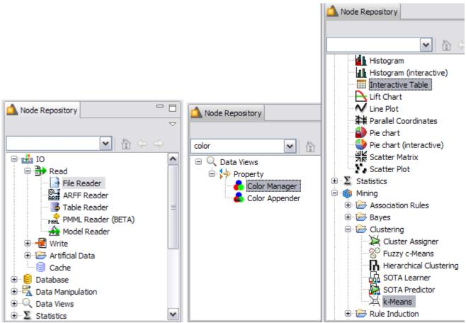
below (left picture) and drag&drop the *File Reader* icon into the *Workflow Editor* window. The next node for now will be the *K-Means* clustering algorithm. Expand the *Mining* category followed by the *Clustering* category, and then drag the *K-Means* node to the flow (picture on the right).
