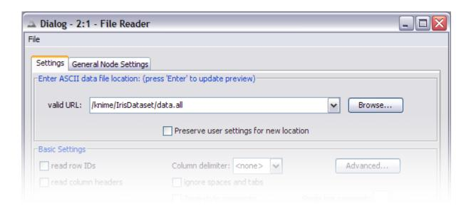
Press OK to close the dialog of the File Reader node. Once the node has been configured correctly, it switches to yellow (meaning ready for execution). After that, the *K-Means* node will immediately turn yellow, since its default settings will be applied. To be sure, that the default settings fit your needs, open the dialog and inspect the default settings.
