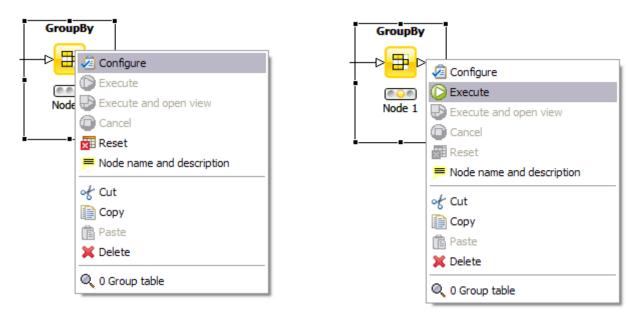
When the dialog is closed by pressing the "OK" button, the node is configured and the status light changes to yellow: the node is ready to be executed. Right-click on the node again shows an enabled "Execute" option; pressing it will execute the node and the result of this node will be available at the out-port. After a successful execution the stauts light of the node is green.
